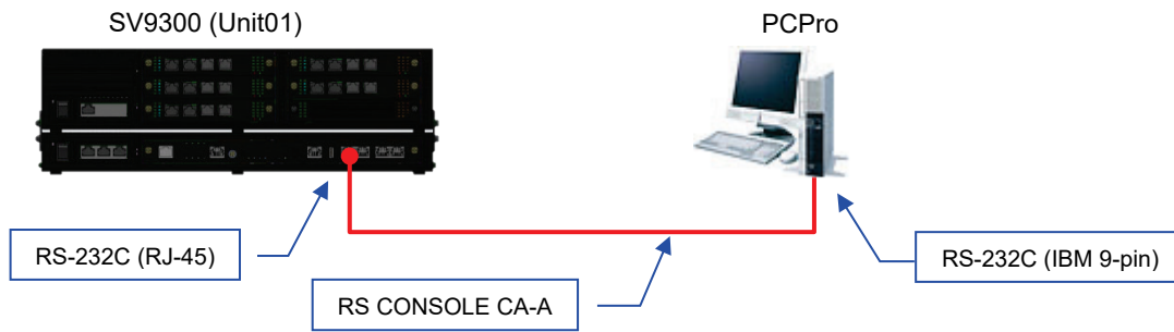
Figure 6-8 PCPro Direct Connection
